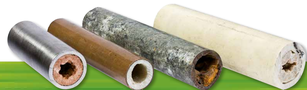
Calcified pipes, from left to right: Stainless steel, copper, iron, plastic;
